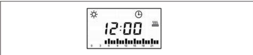
The previous illustration shows the current day. It is indicated in the time axis at the bottom of the the bottom of the illustration that the heater is operating from 5 o'clock in the morning.
