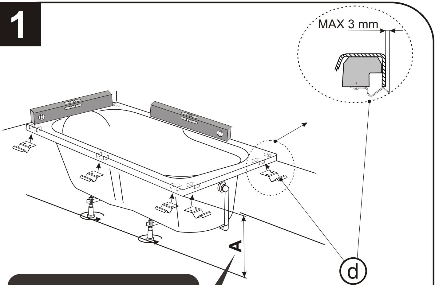
**CZ: Výška panelu****GB: High of panel****D: Höhe der Paneel****F: Hauteur du panneau****RU: Высота панели****2**
