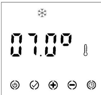
**11.4. 6-order pilot mode:**
